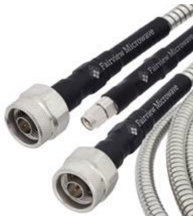
Figure 1.8: Armoring prevents the cable from being bent beyond the specified radius while also mitigating the damage that comes with shear forces and torsional strains. These can be used in precision VNA test cables to protect the thin, delicate coaxial structure beneath
