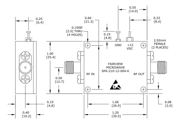
NOTE: HEAT SINK REQUIRED FOR PROPER OPERATION, UNIT IS COOLED BY CONDUCTING TO HEAT SINK.
