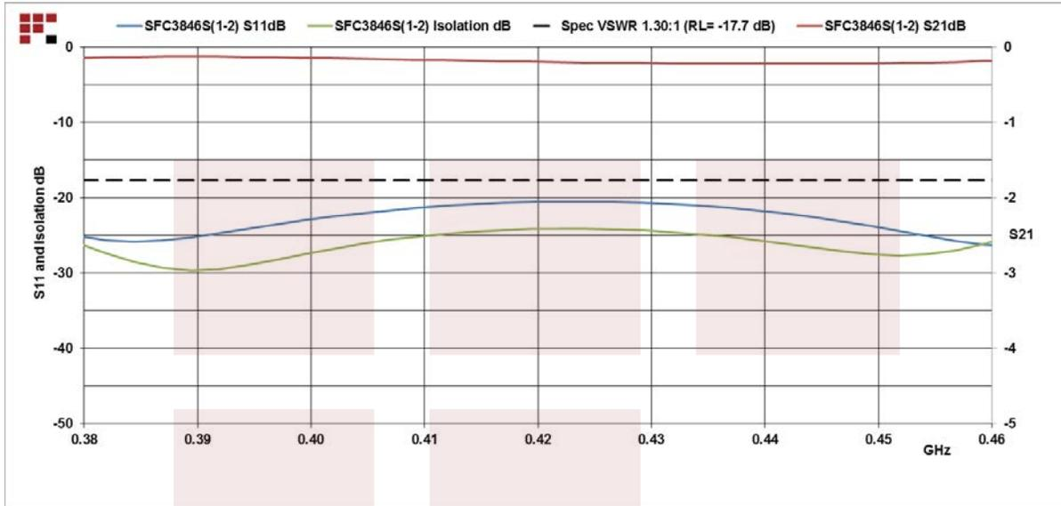
High Power Circulator SMA Female With 20 dB Isolation From 380 MHz to 460 MHz Rated to 1000 Watts from Fairview Microwave is in-stock and available to ship same-day. All of our RF/microwave products are available off-the-shelf from our ISO 9001:2008 certified facilities in Allen, Texas. Fairview Microwave is RF on-demand.
