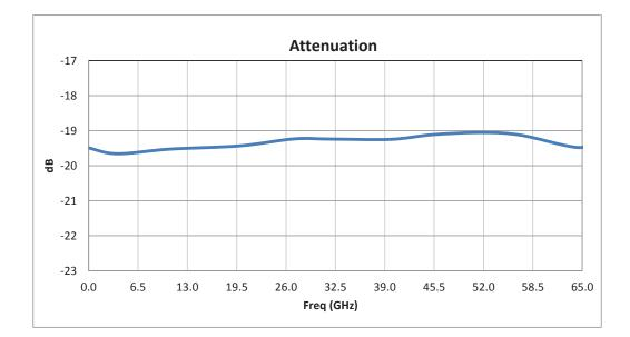
20 dB Fixed Attenuator 1.85mm Male (Plug) to 1.85mm Female (Jack) Up to 65 GHz Rated to 1 Watt, Passivated Stainless Steel Body, 1.65 VSWR
