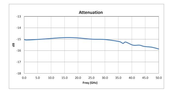
15 dB Fixed Attenuator 2.4mm Male (Plug) to 2.4mm Female (Jack) Up to 50 GHz Rated to 1 Watt, Passivated Stainless Steel Body, 1.75 VSWR
