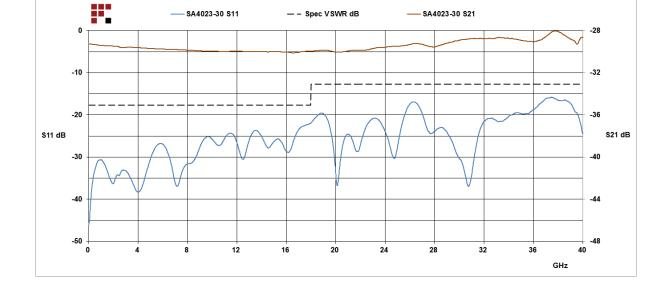
30 dB Fixed Attenuator 2.92mm Male (Plug) to 2.92mm Female (Jack) Directional Up to 40 GHz Rated to 20 Watts, Heatsink Body, 1.4 VSWR from Fairview Microwave is in-stock and available to ship same-day. All of our RF/microwave products are available off-the-shelf from our ISO 9001:2008 certified facilities in Lewisville, Texas. Fairview Microwave is RF on-demand.
