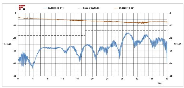
10 dB Fixed Attenuator 2.92mm Male (Plug) to 2.92mm Female (Jack) Directional Up to 40 GHz Rated to 10 Watts, Heatsink Body, 1.4 VSWR from Fairview Microwave is in-stock and available to ship same-day. All of our RF/microwave products are available off-the-shelf from our ISO 9001:2008 certified facilities in Lewisville, Texas. Fairview Microwave is RF on-demand.
