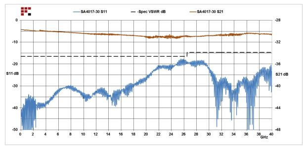
30 dB Fixed Attenuator 2.92mm Male (Plug) to 2.92mm Female (Jack) Up to 40 GHz Rated to 5 Watts, Heatsink Body, 1.45 VSWR from Fairview Microwave is in-stock and available to ship same-day. All of our RF/microwave products are available off-the-shelf from our ISO 9001:2008 certified facilities in Lewisville, Texas. Fairview Microwave is RF on-demand.
