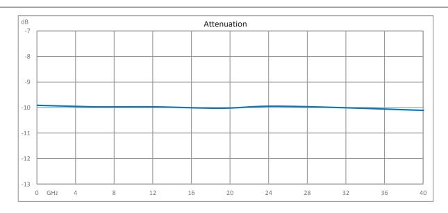
10 dB Fixed Attenuator 2.92mm Male (Plug) to 2.92mm Female (Jack) Up to 40 GHz Rated to 1 Watt, Passivated Stainless Steel Body, 1.4 VSWR from Fairview Microwave is in-stock and available to ship same-day. All of our RF/microwave products are available off-the-shelf from our ISO 9001:2008 certified facilities in Lewisville, Texas. Fairview Microwave is RF on-demand.
