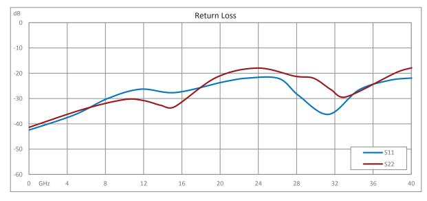
6 dB Fixed Attenuator 2.92mm Male (Plug) to 2.92mm Female (Jack) Up to 40 GHz Rated to 1 Watt, Passivated Stainless Steel Body, 1.4 VSWR
