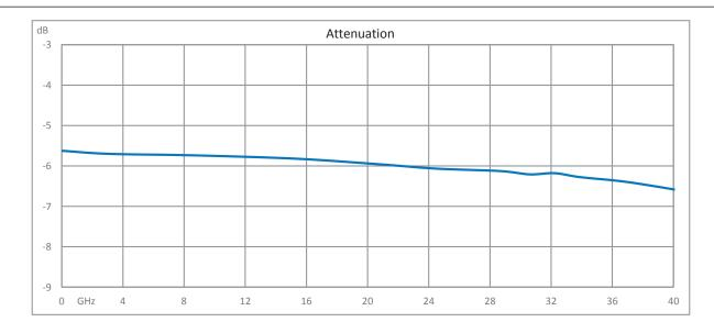
6 dB Fixed Attenuator 2.92mm Male (Plug) to 2.92mm Female (Jack) Up to 40 GHz Rated to 1 Watt, Passivated Stainless Steel Body, 1.4 VSWR from Fairview Microwave is in-stock and available to ship same-day. All of our RF/microwave products are available off-the-shelf from our ISO 9001:2008 certified facilities in Lewisville, Texas. Fairview Microwave is RF on-demand.
