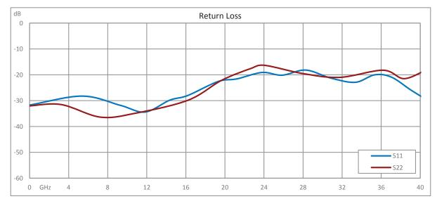
5 dB Fixed Attenuator 2.92mm Male (Plug) to 2.92mm Female (Jack) Up to 40 GHz Rated to 1 Watt, Passivated Stainless Steel Body, 1.4 VSWR
