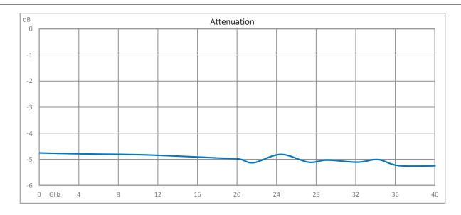
5 dB Fixed Attenuator 2.92mm Male (Plug) to 2.92mm Female (Jack) Up to 40 GHz Rated to 1 Watt, Passivated Stainless Steel Body, 1.4 VSWR from Fairview Microwave is in-stock and available to ship same-day. All of our RF/microwave products are available off-the-shelf from our ISO 9001:2008 certified facilities in Lewisville, Texas. Fairview Microwave is RF on-demand.
