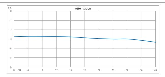
3 dB Fixed Attenuator 2.92mm Male (Plug) to 2.92mm Female (Jack) Up to 40 GHz Rated to 1 Watt, Passivated Stainless Steel Body, 1.4 VSWR from Fairview Microwave is in-stock and available to ship same-day. All of our RF/microwave products are available off-the-shelf from our ISO 9001:2008 certified facilities in Lewisville, Texas. Fairview Microwave is RF on-demand.
