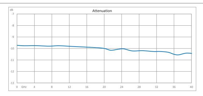
10 dB Fixed Attenuator 2.92mm Male (Plug) to 2.92mm Female (Jack) Up to 40 GHz Rated to 0.5 Watts, Passivated Stainless Steel Body, 1.5 VSWR from Fairview Microwave is in-stock and available to ship same-day. All of our RF/microwave products are available off-the-shelf from our ISO 9001:2008 certified facilities in Lewisville, Texas. Fairview Microwave is RF on-demand.
