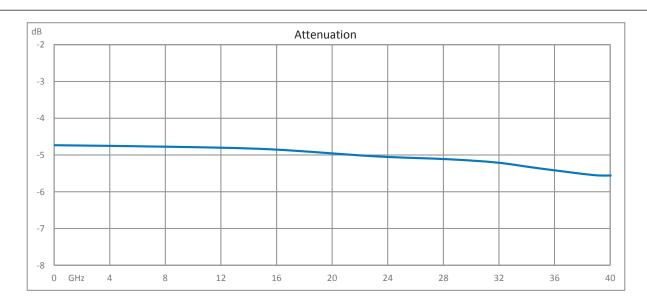
5 dB Fixed Attenuator 2.92mm Male (Plug) to 2.92mm Female (Jack) Up to 40 GHz Rated to 0.5 Watts, Passivated Stainless Steel Body, 1.5 VSWR from Fairview Microwave is in-stock and available to ship same-day. All of our RF/microwave products are available off-the-shelf from our ISO 9001:2008 certified facilities in Lewisville, Texas. Fairview Microwave is RF on-demand.
