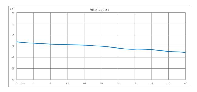
3 dB Fixed Attenuator 2.92mm Male (Plug) to 2.92mm Female (Jack) Up to 40 GHz Rated to 0.5 Watts, Passivated Stainless Steel Body, 1.5 VSWR from Fairview Microwave is in-stock and available to ship same-day. All of our RF/microwave products are available off-the-shelf from our ISO 9001:2008 certified facilities in Lewisville, Texas. Fairview Microwave is RF on-demand.
