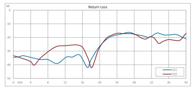
3 dB Fixed Attenuator 2.92mm Male (Plug) to 2.92mm Female (Jack) Up to 40 GHz Rated to 0.5 Watts, Passivated Stainless Steel Body, 1.5 VSWR
