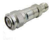
10 dB Fixed Attenuator TNC Male (Plug) to TNC Female (Jack) Up to 3 GHz Rated to 1 Watt, Brass Tri-Metal Body, 1.25 VSWR
