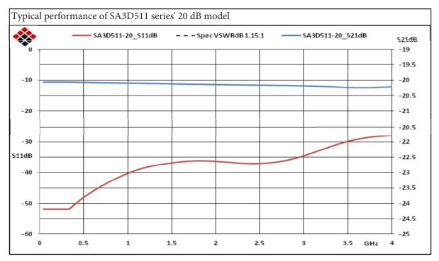
20 dB Fixed Attenuator 7/16 Male (Plug) to 7/16 Female (Jack) Up to 3 GHz Rated to 50 Watts, Heatsink Body, 1.15 VSWR from Fairview Microwave is in-stock and available to ship same-day. All of our RF/microwave products are available off-the-shelf from our ISO 9001:2008 certified facilities in Lewisville, Texas. Fairview Microwave is RF on-demand.
