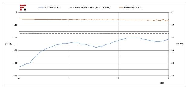
10 dB Fixed Attenuator 7/16 Male (Plug) to 7/16 Female (Jack) Up to 3 GHz Rated to 100 Watts, Heatsink Body, 1.3 VSWR
