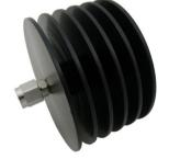
30 dB Fixed Attenuator 3.5mm Male (Plug) to 3.5mm Female (Jack) Up to 28 GHz Rated to 25 Watts, Heatsink Body, 1.35 VSWR
