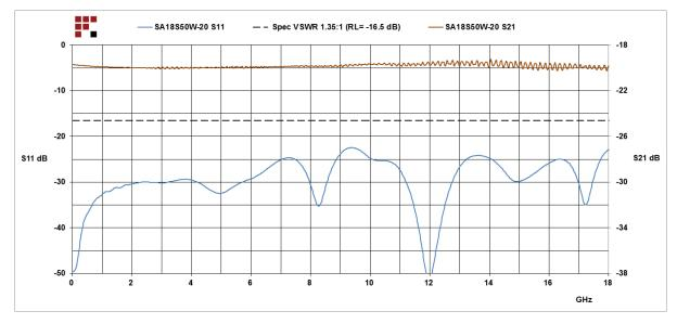
20 dB Fixed Attenuator SMA Male (Plug) to SMA Female (Jack) Up to 18 GHz Rated to 50 Watts, Heatsink Body, 1.35 VSWR
