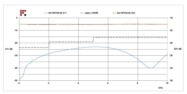
20 dB Fixed Attenuator SMP Male (Plug) to SMP Female (Jack) Up to 10 GHz Rated to 2 Watts, Passivated Stainless Steel Body, 1.4 VSWR from Fairview Microwave is in-stock and available to ship same-day. All of our RF/microwave products are available off-the-shelf from our ISO 9001:2008 certified facilities in Lewisville, Texas. Fairview Microwave is RF on-demand.
