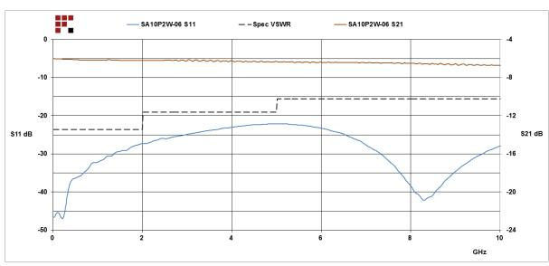
6 dB Fixed Attenuator SMP Male (Plug) to SMP Female (Jack) Up to 10 GHz Rated to 2 Watts, Passivated Stainless Steel Body, 1.4 VSWR from Fairview Microwave is in-stock and available to ship same-day. All of our RF/microwave products are available off-the-shelf from our ISO 9001:2008 certified facilities in Lewisville, Texas. Fairview Microwave is RF on-demand.
