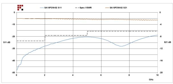
2 dB Fixed Attenuator SMP Male (Plug) to SMP Female (Jack) Up to 10 GHz Rated to 2 Watts, Passivated Stainless Steel Body, 1.4 VSWR from Fairview Microwave is in-stock and available to ship same-day. All of our RF/microwave products are available off-the-shelf from our ISO 9001:2008 certified facilities in Lewisville, Texas. Fairview Microwave is RF on-demand.
