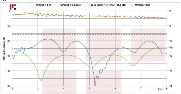
4 Way Power Divider SMA Connectors From 2 GHz to 8 GHz Rated at 30 Watts from Fairview Microwave is in-stock and available to ship same-day. All of our RF/microwave products are available off-the-shelf from our ISO 9001:2008 certified facilities in Allen, Texas. Fairview Microwave is RF on-demand.
