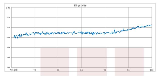
30 dB WR-112 Waveguide Crossguide Coupler with UG-51/U Square Cover Flange and N Female Coupled Port from 7.05 GHz to 10 GHz in Bronze from Fairview Microwave is in-stock and available to ship same-day. All of our RF/microwave products are available off-the-shelf from our ISO 9001:2008 certified facilities in Allen, Texas. Fairview Microwave is RF on-demand.
