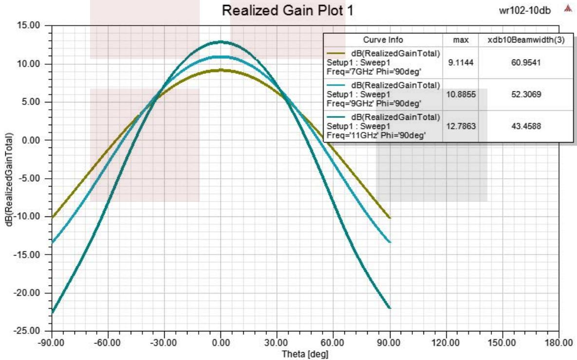
WR-102 Standard Gain Horn with 10 dBi gain, End Launch SMA Female connector from Fairview Microwave is in-stock and available to ship same-day. All of our RF/microwave products are available off-the-shelf from our ISO 9001:2008 certified facilities in Lewisville, Texas. Fairview Microwave is RF on-demand.
