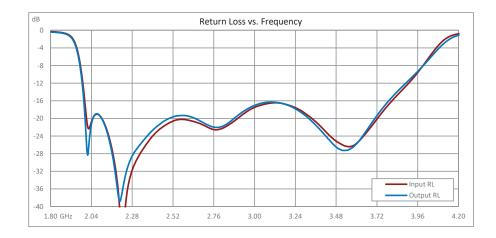
Bandpass Cavity Filter Operating from 2.1 GHz to 3.8 GHz with a 2 GHz Passband Bandwidth with SMA Female Connectors from Fairview Microwave is in-stock and available to ship same-day. All of our RF/microwave products are available off-the-shelf from our ISO 9001:2008 certified facilities in Lewisville, Texas. Fairview Microwave is RF on-demand.
