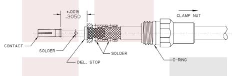
3. INSERT CABLE/ CONTACT SUB-ASSEMBLY UNTIL SEATED AND TIGHTEN CLAMP NUT TO 25-35 IN-LBS.
