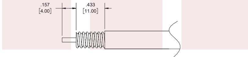
2. SLIDE INSULATOR ③ OVER CABLE CENTER CONDUCTOR. INSERT CENTER CONTACT AND SOLDER. WRAP THE CABLE BY SOLDER WIRE.
