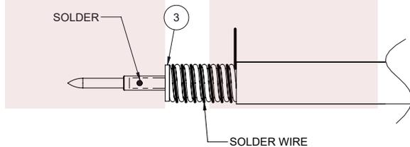
3. PUSH THE CONNECTOR BODY INTO THE CABLE, UNTIL IT STOPS. SOLDER THE CONNECTOR BODY WITH CABLE AND COVER HEATSHRINK SLEEVE.
