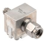
20 dB Fixed Attenuator 1.0mm Male (Plug) to 1.0mm Female (Jack) Up to 110 GHz Rated to 0.5 Watts Passivated Stainless Steel Body 1.8:1 VSWR
