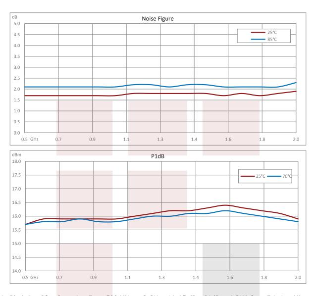
50 dB Gain Block Amplifier Operating From 500 MHz to 2 GHz with 15 dBm P1dB and SMA from Fairview Microwave is instock and available to ship same-day. All of our RF/microwave products are available off-the-shelf from our ISO 9001:2008 certified facilities in Allen, Texas. Fairview Microwave is RF on-demand.
