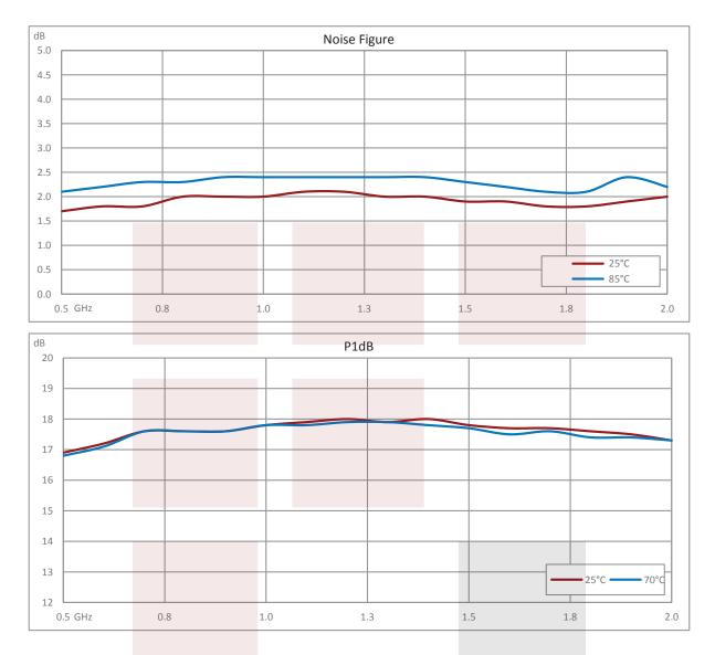
17 dB Gain Block Amplifier Operating From 500 MHz to 2 GHz with 15 dBm P1dB and SMA from Fairview Microwave is instock and available to ship same-day. All of our RF/microwave products are available off-the-shelf from our ISO 9001:2008 certified facilities in Allen, Texas. Fairview Microwave is RF on-demand.
