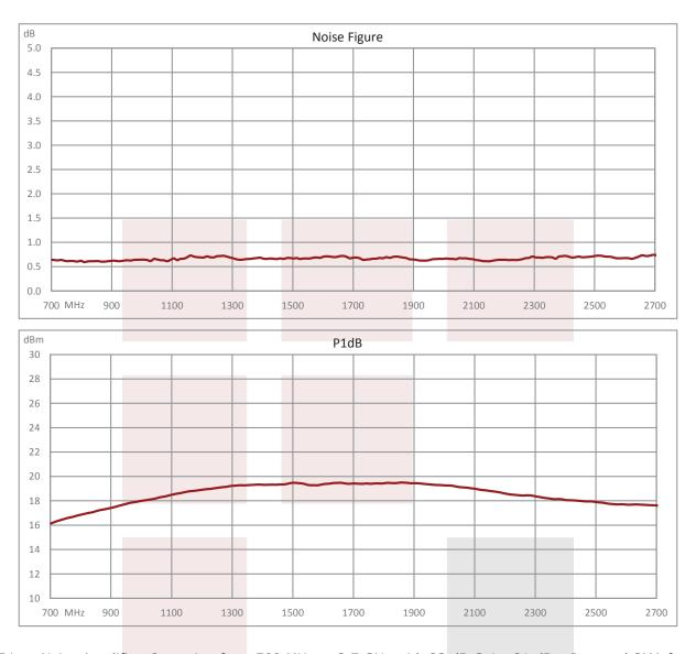
0.7 dB NF Low Noise Amplifier, Operating from 700 MHz to 2.7 GHz with 23 dB Gain, 21 dBm Psat and SMA from Fairview Microwave is in-stock and available to ship same-day. All of our RF/microwave products are available off-the-shelf from our ISO 9001:2008 certified facilities in Lewisville, Texas. Fairview Microwave is RF on-demand.
