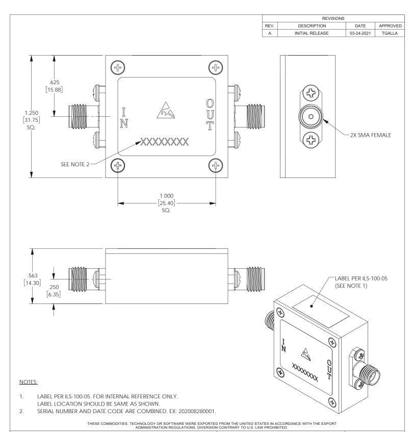
UNLESS OTHERWISE SPECIFIED LEADING DIMENSIONS ARE INCHES DIMENSIONS IN [] ARE MILLIMETERS THIRD-ANGLE PROJECTION Fairview Microwave  $\oplus \ \circlearrowleft$ TOLERANCES: CABLE LENGTH (L) TOLERANCES: THE INFORMATION AND
