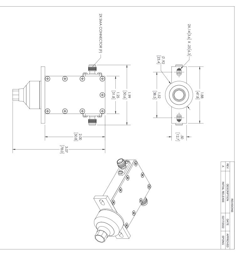
Fairview Microwave A  $X = \pm .2$  [5.08] FRACTIONS  $XX = \pm .02$  [.51]  $\pm .1/32$   $.XXX = \pm .005$  [.13] ANGLES  $\pm .1^{\circ}$ CAGE CODE 3FKR5 ALL DIMENSIONS SHOWN ARE FOR REFERENCE ONLY. TOLERANCES: L ≤ 12 [305] = +1 [25] / -0
